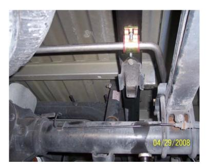
Installing a 402 U-Bolt Detail
